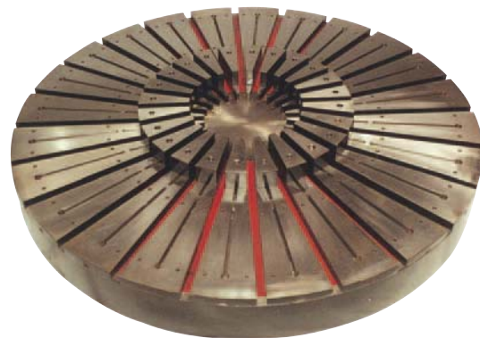
Axial Clamping - can machine OD or ID at a time.
