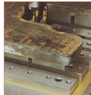
Side milling can be performed using raised blocks for free cutter movement.
