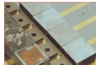
Number of small components can be machined using simple pole extension fixtures.
